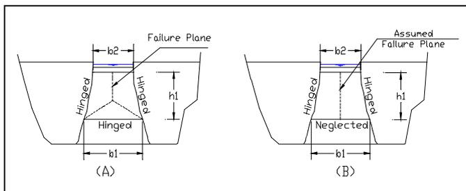
Figure 9: Bending Failure of the clay core
