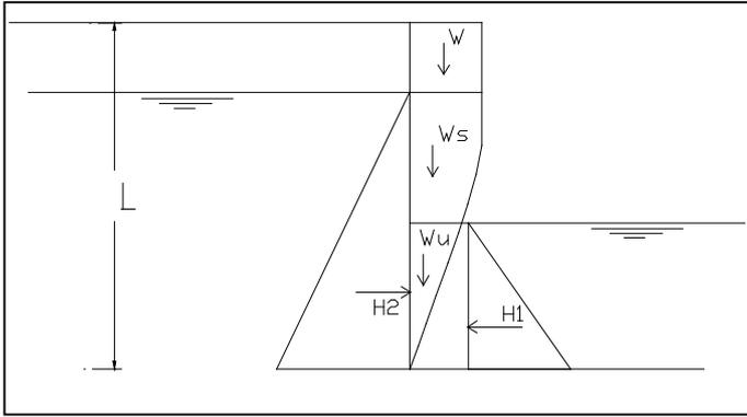
Figure 4: Forces for shear failure.
