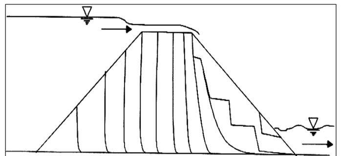
Figure 6: Headcut advance mechanism (Hanson et al, 2000)
