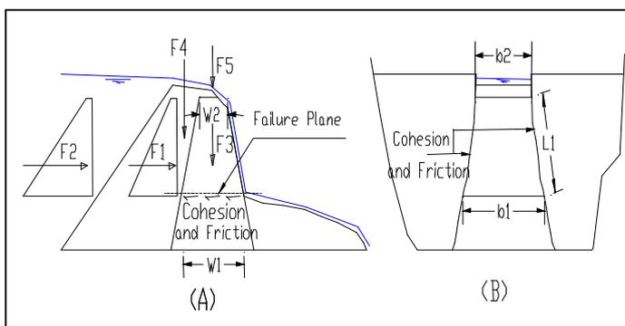
Figure 7: Forces acting on the clay core wall.
