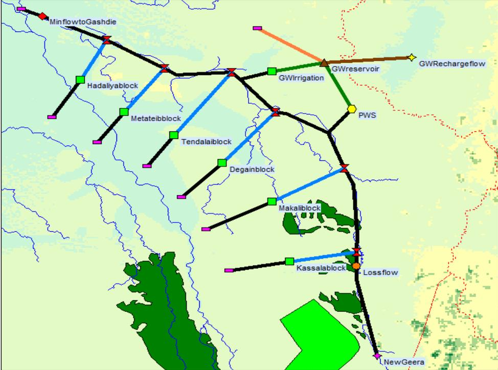
Fig 4: Schematization of surface and groundwater of Gash.
