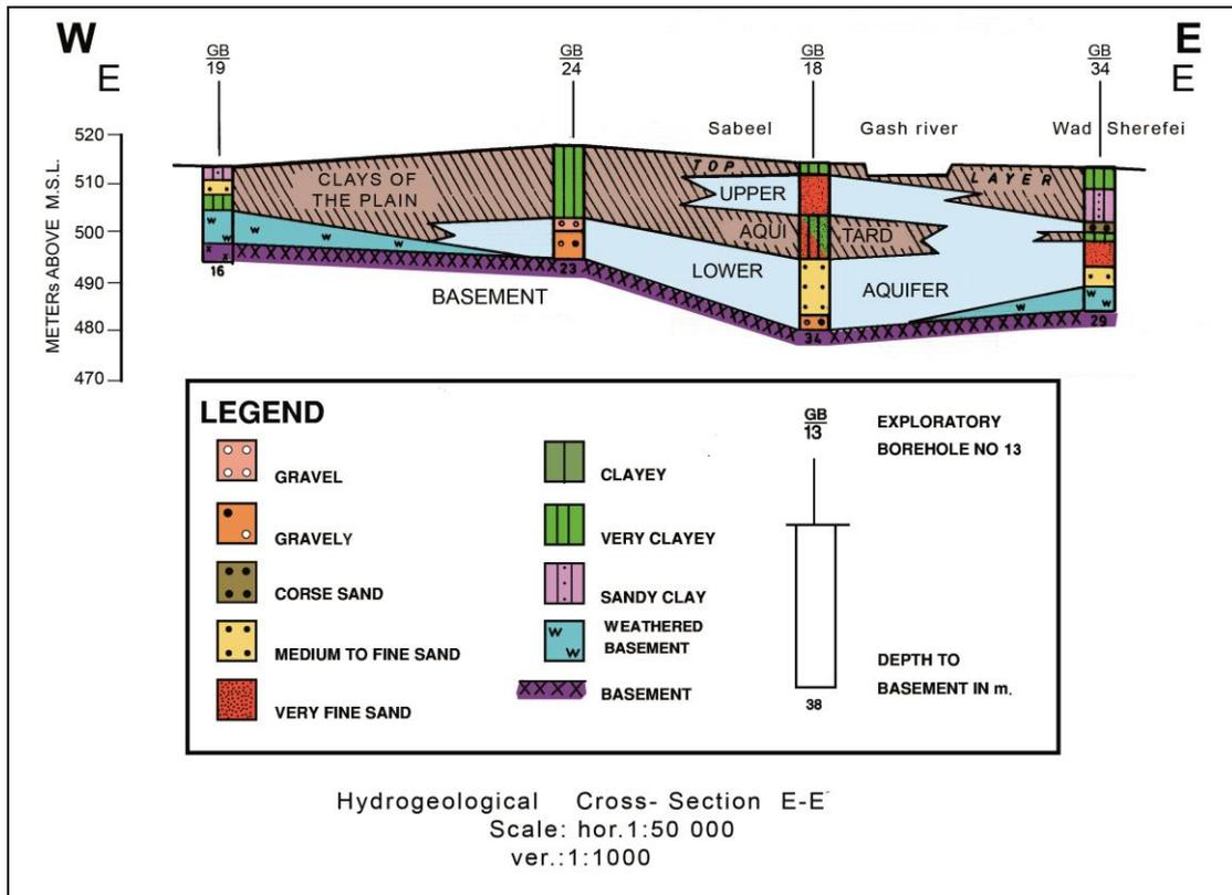
Fig 1: Example of cross-sections defining the aquifer geometry.
