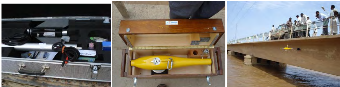
Fig (7): current-meter instruments used at Kassala Bridge Gauging Station
