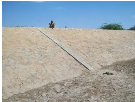
Fig (3): Inclined gauge staff placed upon the right bank of New Geera gauging station
