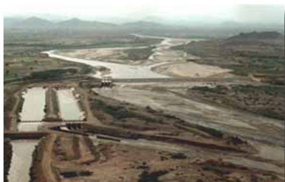
Figure 1: A single intake is used to irrigate 18,000 ha of Yemen's Wadi Mawr scheme (Source: Mehari Haile et al., 2005)
